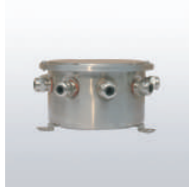
AVX105 Waterproof Stainless steel box IP68 Imported silicon rubber ring Mounted with 1pc M20 and 9pcs M16 cable glands max 12V/150W and 12V/300W transformer is capable to be fit in
