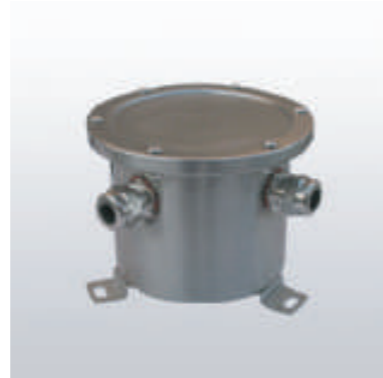
AVX104 Waterproof Stainless steel box IP68 Imported silicon rubber ring Mounted with 8pcs M20 cable glands max 12V/50W and 12V/100W transformer is capable to be fit in
