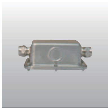
AVX102 Waterproof Stainless steel box IP68 Imported silicon rubber ring Mounted with 6pcs M20 cable glands max
