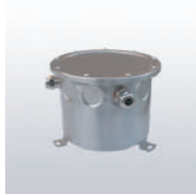
AVX106 Waterproof Stainless steel box IP68 Imported silicon rubber ring Mounted with 1pcs M20 cable glands max, and 9pcs M16 cable glands max
